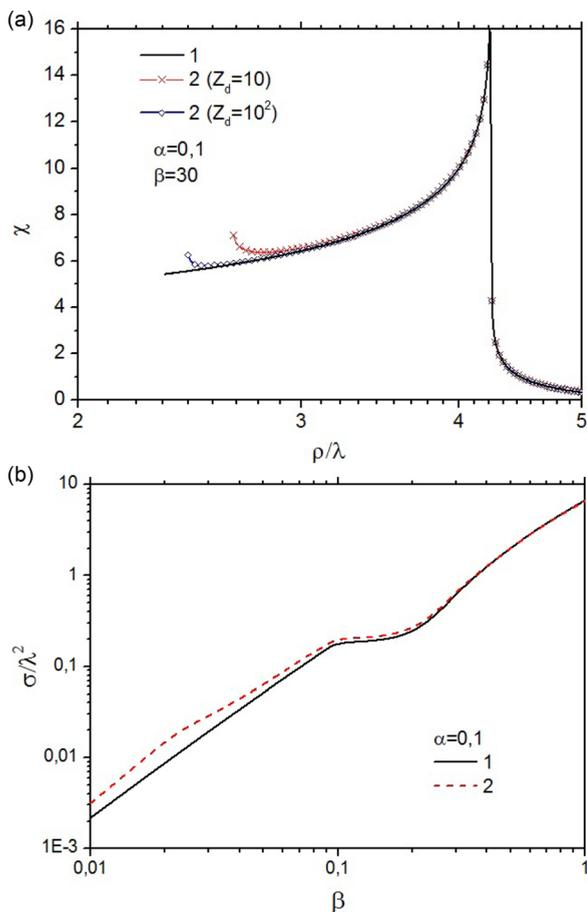
FIG. 3. In (a), the scattering angle obtained using the Yukawa potential (line 1) and the interaction potential (5) of the ion with the spherical dust grain (line 2). In Figure 3(b), the scattering cross section obtained using the Yukawa potential (line 1) and the interaction potential (5) of the ion with the spherical dust grain (line 2) is shown.
