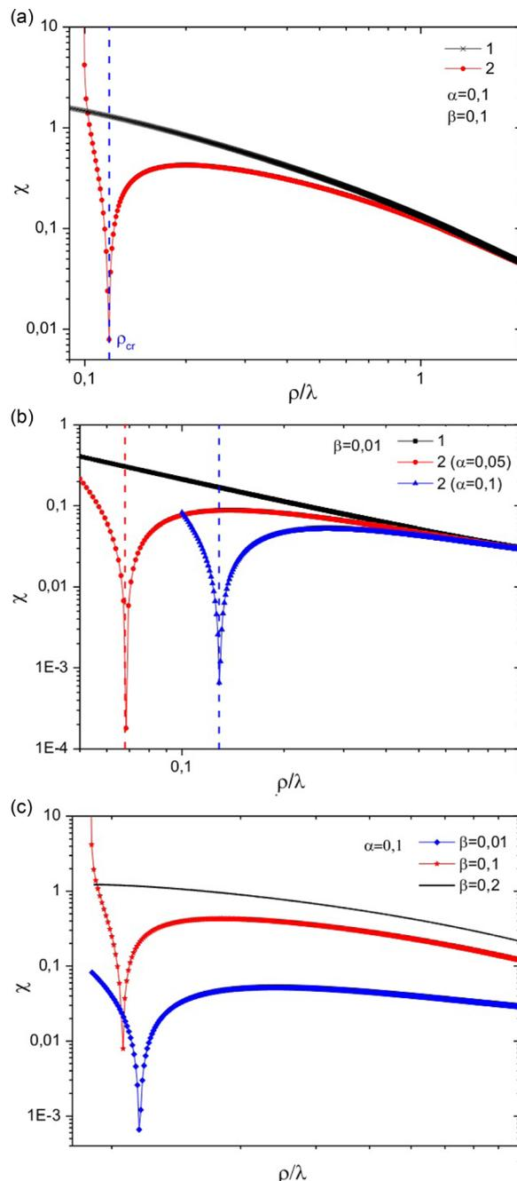
FIG. 5. In (a) and (b), the dust particle-dust particle scattering angle obtained using the Yukawa potential (line 1) and the dust particle-dust particle interaction potential (13) (line 2), which takes into account an induced dipole moment, is shown. In Figure 4(c), the scattering angle obtained using the dust particle-dust particle interaction potential (13) for the different values of  $\beta$  is given.
