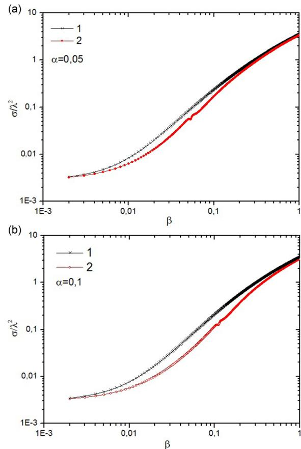
FIG. 7. The scattering cross section obtained using the Yukawa potential (line 1) and the interaction potential (13) (line 2) taking into account an induced dipole moment.
