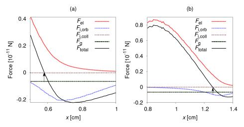
Fig. 3 Spatial dependence of the different force components, for conditions L = 25 mm,  $V_{\text{pp}} = 150 \text{ V}$  at p = 10 Pa,  $V_{\text{DC}} = 0 \text{ V}$  (a) and  $V_{\text{DC}} = -90 \text{ V}$  (b).
