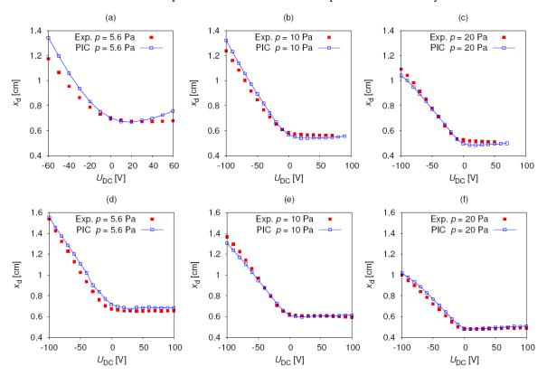
Fig. 4 Equilibrium position of the dust layer as a function of the DC bias,  $V_{\rm DC}$ , for conditions:  $V_{\rm pp} = 150$  V at p = 5.6 Pa, p = 10 Pa, p = 20 Pa, L = 25 mm (upper row) and L = 36 mm (lower row).
