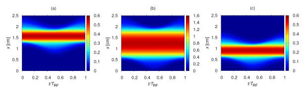
Fig. 2 Effect of DC bias on the spatio-temporal distribution of the electron density for L = 25 mm,  $V_{\rm PP} = 150$  V at p = 10 Pa with (a)  $V_{\rm DC} = -90$  V, (b) 0 V, and (c) 90 V. The color scales are given in unites of  $10^9$  cm<sup>-3</sup>.
