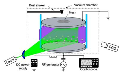
Fig. 1 Scheme of the experimental setup.
