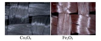
Fig. 1 Optical microscope photographs of glasscloth with  $Co_3O_4$  and  $Fe_2O_3$
