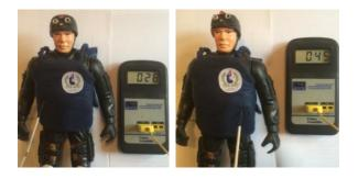
Fig. 5 Before and after heating the jacket of soldier based on glass-cloth with CNT
