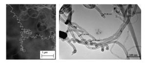
Fig. 3 SEM and TEM images of carbon nanotubes grown on glass-cloth with  $Fe_2O_3$  (2 wt. %)
