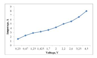
Fig. 4 Current-voltage characteristics of the sample of CNT@glass-cloth
