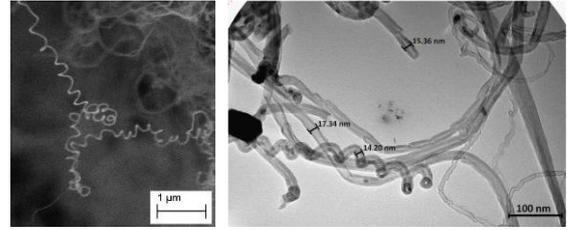
Fig. 3 SEM and TEM images of carbon nanotubes grown on glass-cloth with Fe<sub>2</sub>O<sub>3</sub> (2 wt. %)
