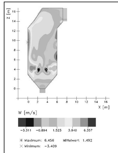
Fig.4 The distribution component of the velocity V in longitudinal section and the height of the combustion chamber
