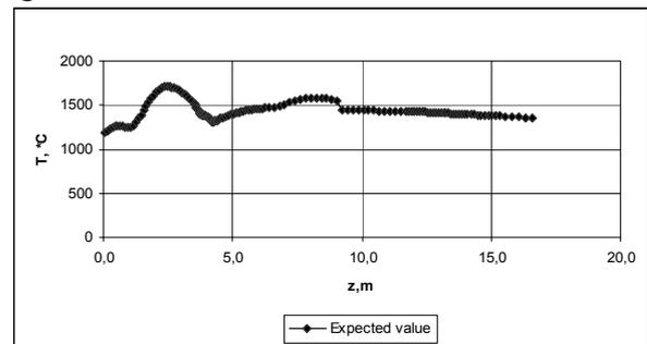
Fig.8 The temperature distribution on the height of the combustion chamber
