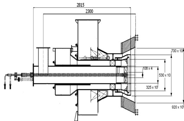
Fig.2 The general form of the combustion chamber and coal-dust burner
