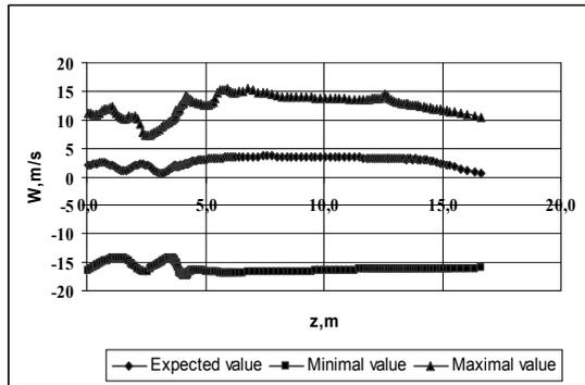
Fig.5 The distribution of the velocity component W in the burner section and the height of the combustion chamber
