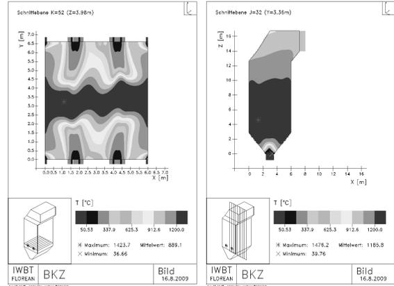
Fig.7 The temperature profile of the burners and in the longitudinal section of the combustion chamber
