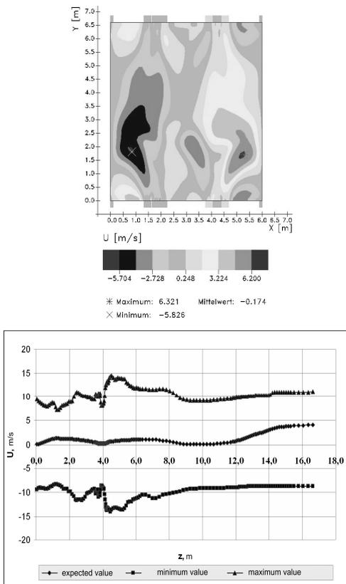
Fig.3 The distribution of the velocity component U in the burner section on the height of the combustion chamber
