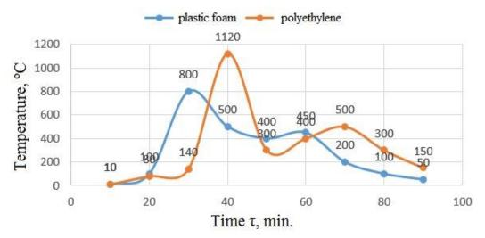
Figure 4. The temperature profile of the combustion of briquettes with polyethylene and foam
