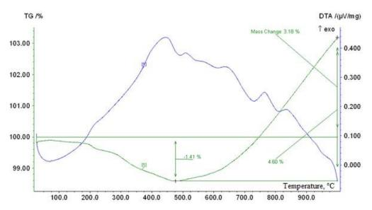
Figure 3. Thermogravimetric curve of the decomposition of coal with polyethylene
