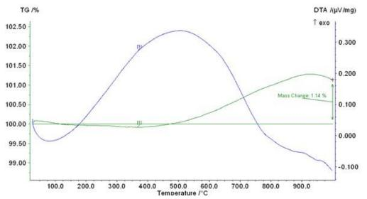
Figure 2. Thermogravimetric curve of the decomposition of the briquette with foam
