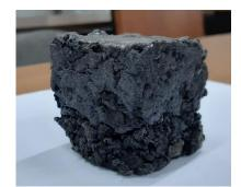
Figure 1. The appearance of the resulting coal briquette
