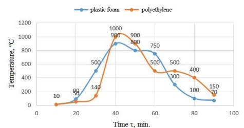
Figure 6. Burning temperature profile of briquettes with polyethylene and foam in the presence of 10% clay
