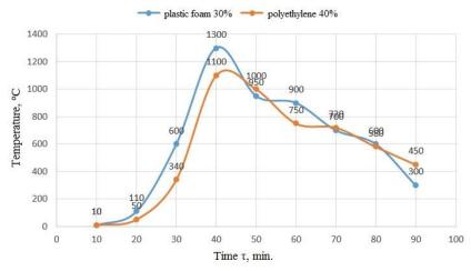
Figure 7. The combustion temperature profile of briquettes with 40% polyethylene and 30% polystyrene in the presence of 30% clay
