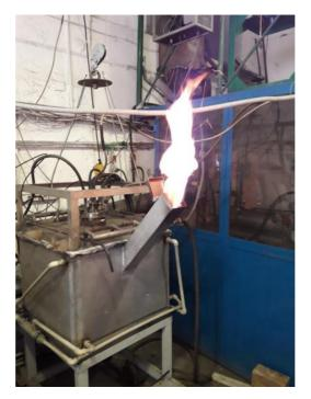
Figure 6. Photo of the combustible gas control flame from the pipe for supplying of briquetted WW.
