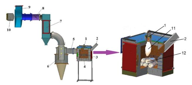
Figure 4. Layout of the experimental unit for plasma gasification of WW and scheme of the plasma reactor: 1 - arc plasmatron; 2 - pipe for supplying of briquetted WW; 3 - WW gasification zone; 4 - reactor; 5 - chamber for combustible gas removal from the reactor; 6 - cyclone combustion chamber; 7 - gas purification unit with a bag filter; 8 - control valve; 9 - ventilator of exhaust system; 10 - engine of the exhaust system; 11 - plasma flame; 12 - WW briquettes.
