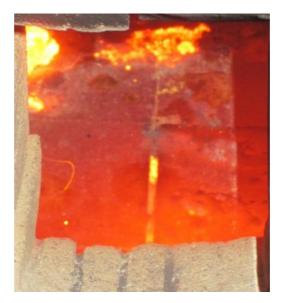
Figure 7. Photo of hot ash on the bottom of the reactor after plasmatron turn off.
