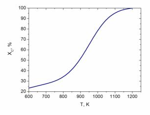
Figure 2. Carbon gasification degree dependence on temperature of WW gasification.
