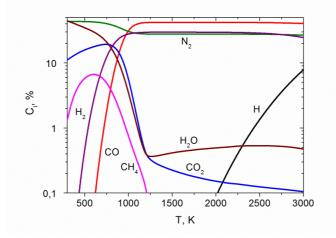
Figure 1. Variation in concentration of gaseous components depending on the temperature of WW air gasification.
