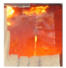
Figure 8. Photo of hot ash on the bottom of the reactor after plasma torch turn off.
