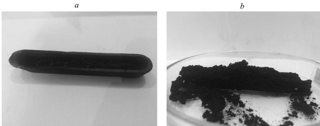
Fig. 2. Catalyst before (a) and after the CVD method use (b).
