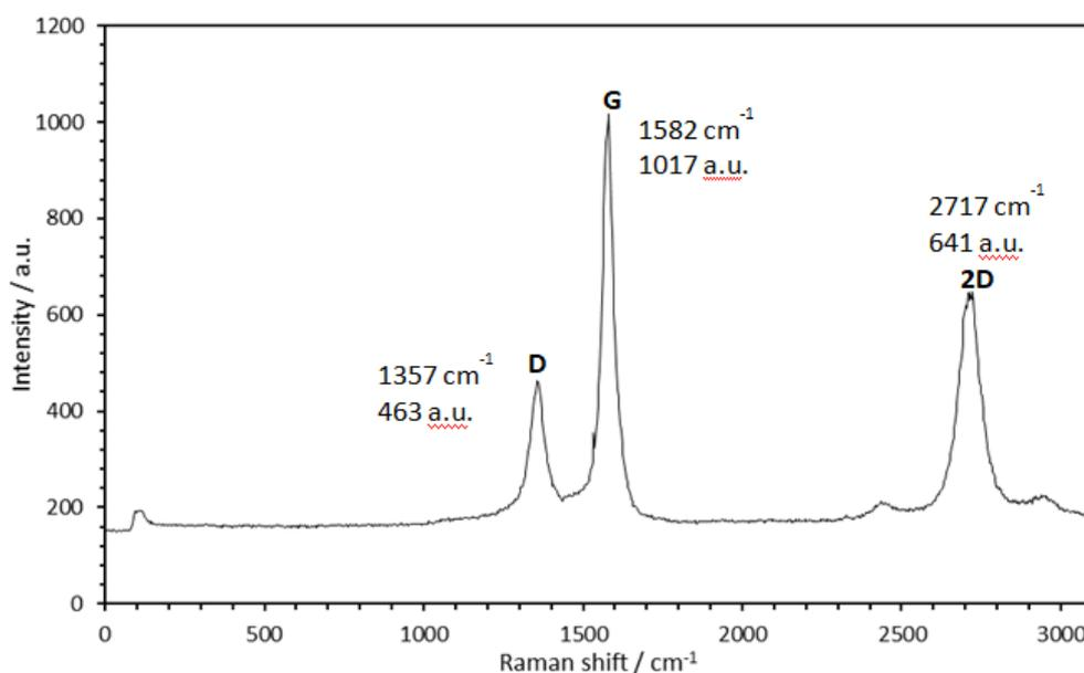
Figure 1 Raman spectra of ARH, showing the three significant peaks (*D*, *G*, *2D*) for the presence and evaluation of graphene layers
