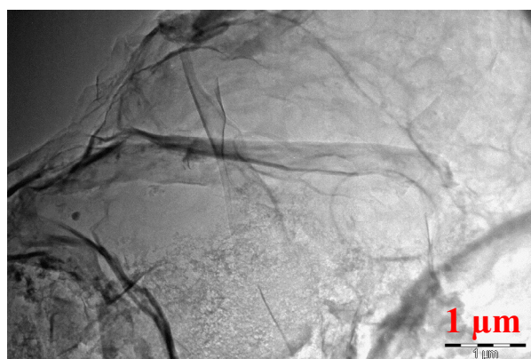
Figure 7 – TEM microimages of the graphene layers
