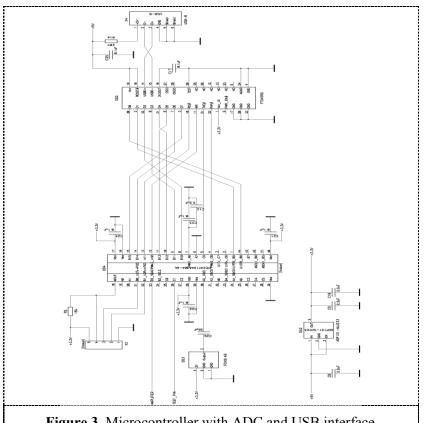
Figure 3. Microcontroller with ADC and USB interface.
