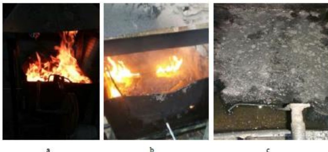
Figure 3 – Formation and use of innovative reagent formulations as a sorbent for the elimination of oil in a pilot plant: a) burning of oil on the water surface with different reagent compositions in the pilot plant; b) formation of thermogranite and reduction of combustion; c) adsorption of petroleum products
