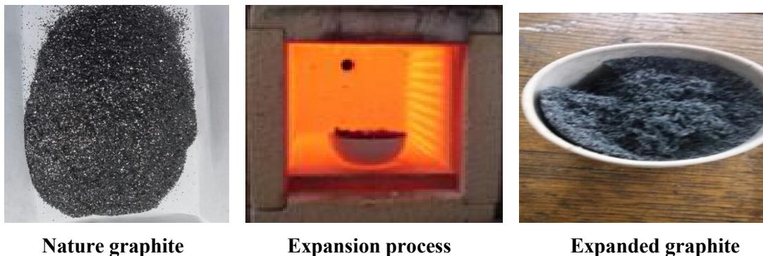
**Figure 2.** Schematic illustration of formation of EG and the synthesis.
