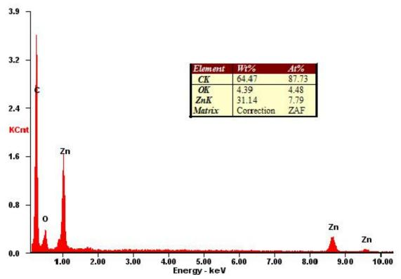
Figure 5. Microanalysis of expanded graphite.
