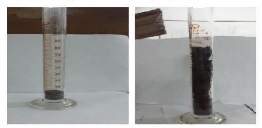
Figure 3. a) mechanical mix before heat treatment b) obtained porous mix after heat treatment.
