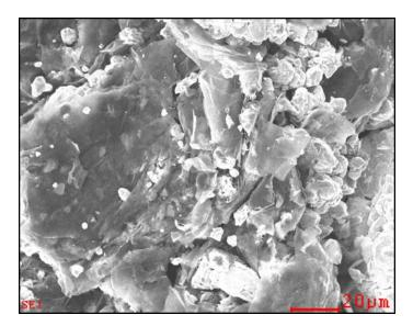
Figure 6. SEM micrograph of expanded graphite.
