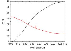
Figure 3. Gas phase components concentrations along the PFS.
