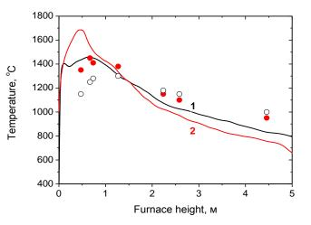
Figure 5. Temperature fields along the furnace height in the central section for conventional (a) and plasma supported (b) regimes.
