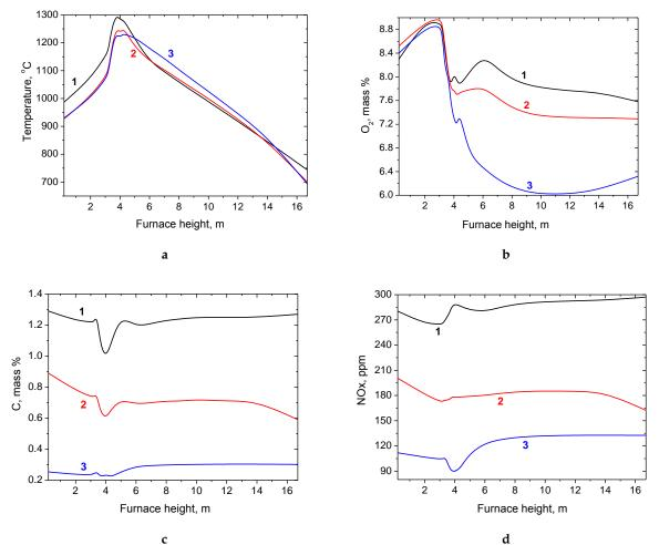
Figure 10. Furnace height distribution of mass average temperature (a), oxygen (b), carbon (c) and NOx (d) mean concentrations: 1-standard operational regime; 2-plasma operational regime with two PFS; 3-plasma operational regime with four PFS.
