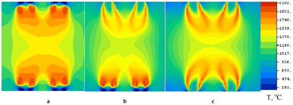
Figure 9. Temperature field within the combustion chamber at the level of the pulverized coal burners: a standard operational regime; b - plasma operational regime with two PFS; c - plasma operational regime with four PFS.
