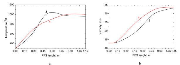
Figure 2. Gas (1) and particles (2) temperatures (a) and velocities (b) along the PFS.
