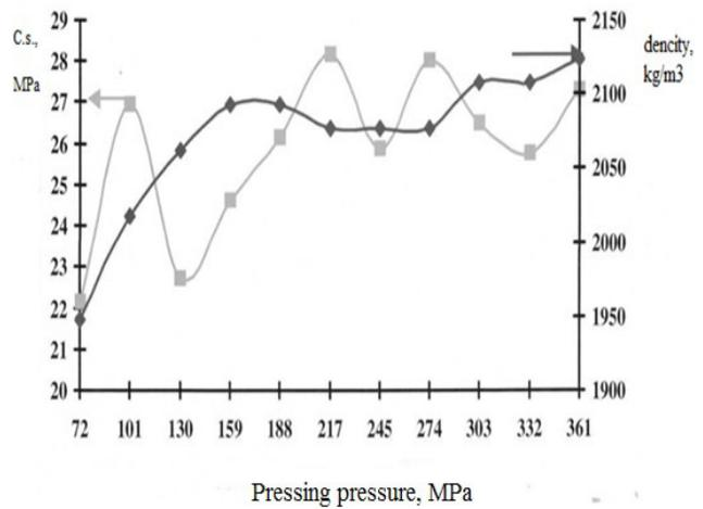
Fig. 10. The dependence of the density and the compressive strength (C.s.) of the pressing pressure in the model system KNO<sub>3</sub> - coal tar.
