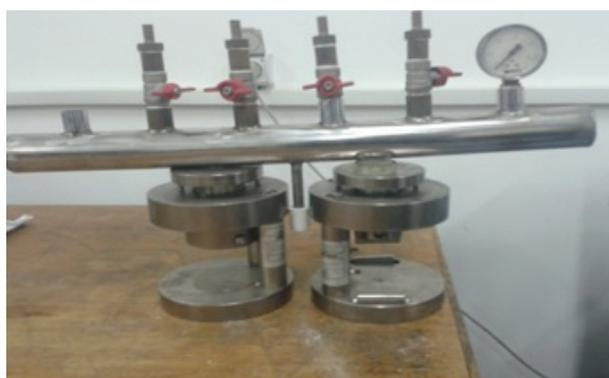
Fig. 2. Installation for determining of gas pressure.
