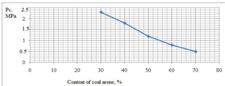
Fig. 6. Influence of the content of coal arenes in the binary mixture of ammonium nitrate - coal arenes on the maximum pressure in the chamber.
