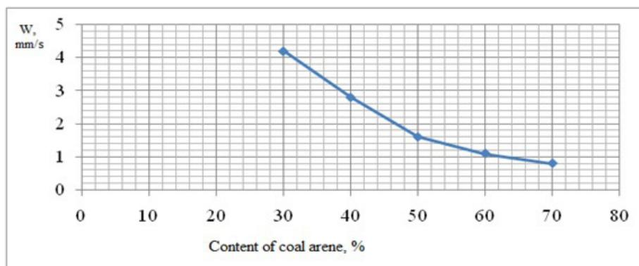
Fig. 5. Influence of the content of coal arenes in the binary mixture of ammonium nitrate - coal arenes on the combustion rate.
