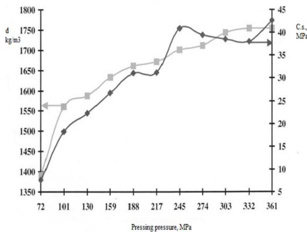
Fig. 9. The dependence of the density (d) and the compressive strength (C.s.) of the pressing pressure in the system KNO<sub>3</sub> - Mg - smokeless powder - coal tar.
