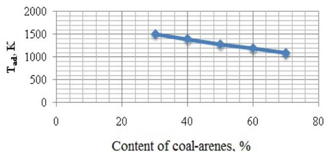
Fig. 3. Influence of the content of coal arenes in a binary mixture of ammonium nitrate - coal arenes on the adiabatic temperature of combustion.
