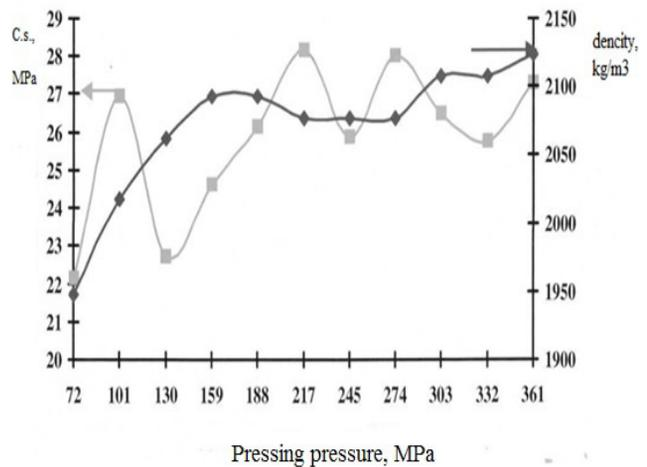
Fig. 10. The dependence of the density and the compressive strength (C.s.) of the pressing pressure in the model system KNO<sub>3</sub> - coal tar.
