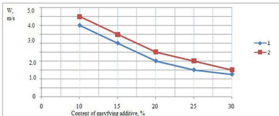
Fig. 7. The dependence of the combustion rate on the content of gasifying additive in the ternary mixture of ammonium nitrate - coal arenes - gasifying additive (1 - polyvinyl alcohol, 2 - melamine).
