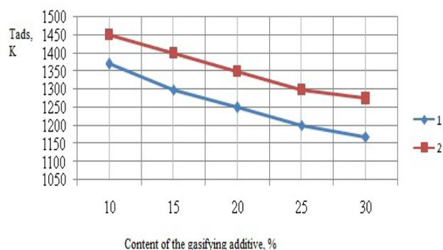
Fig. 4. The dependence of the adiabatic combustion temperature from the content of the gasifying additive in the triple mixture of ammonium nitrate - coal arene - gasifying agent (1 - dicyandiamide, 2 - melamine).
