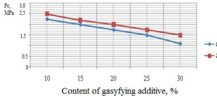
Fig. 8. The dependence of the maximum pressure in the chamber (Pc) on the content of the gasifying additive in the ternary mixture of ammonium nitrate - coal arenes - gasifying additive (1 - polyvinyl alcohol, 2 - melamine).
