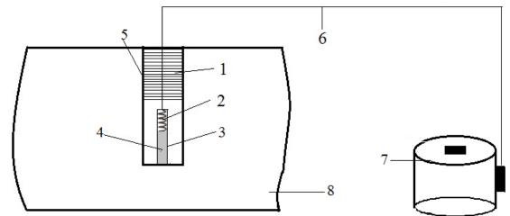
Fig.-1: Experimental Scheme: 1 - quickly grasp mixture (cement + CaCl<sub>2</sub>); 2 - filament of incandescence; 3- gas generator cartridge; 4- pyrotechnic gas-generator composition; 5-blast hole; 6 - cable; 7 – the laboratory autotransformer; 8 - stone
