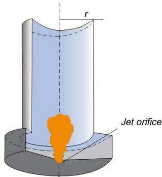
**Figure 1.** The general view of the combustion chamber
