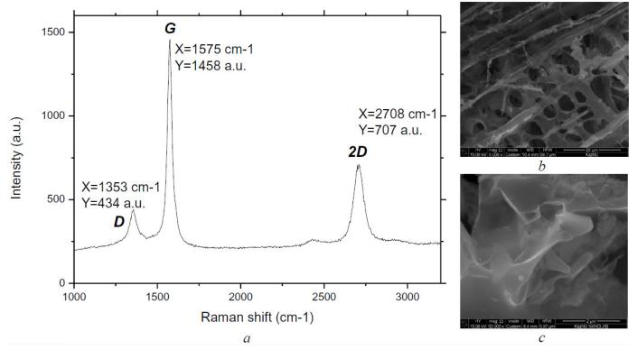
**Figure 1** (a) Raman spectrum of a multilayer graphene and SEM microimages of the graphene film on areas of (b) 60 μm×50 μm and (c) 6 μm×5 μm.
