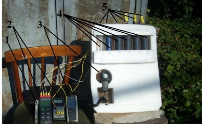
Fig. 2. General view of devices and instruments in the experimental study of solar collectors models: 1 – thermometer, temperature fixing air, 2 – thermometers, temperature fixing water 3 – a device for measuring the intensity of solar radiation, 4 – samples of solar collectors with different absorbing coating, 5 – ChA thermocouple
