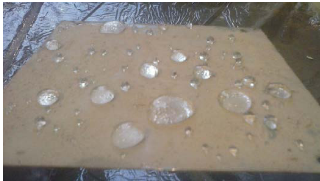
Fig. 2. Photo shows the behavior of water droplets on the surface of the resulting anti-icing coating.
