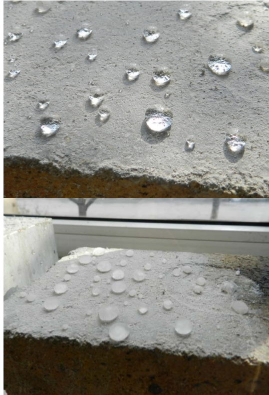
Fig. 3. shows the behavior of water drops at the surface of anti-icing coating is applied to brick.
