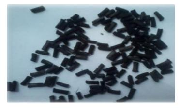
Figure 2 - Granular carbon sorbent from RH and lignosulfonate
