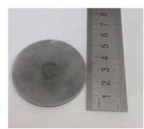
Figure 1 - Solid oxide target for pulsed laser deposition
