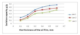
**Fig.3.** Dependence of the sorption capacity of the sorbent on the thickness of the oil film: 1 - rubber foam + carbonizate of sunflower husk (FRCRH- 300); 2-polystyrene foam + carbonizate of rice husk (FPCRH - 400); 3- modified rubber foam (MFR-300)
