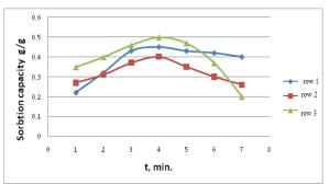
**Fig.2.** Dependence of the sorption capacity of the sorbents on the sorption duration: 1 - rubber foam + carbonizate of sunflower husk (FRCSH- 300) ; 2 - polystyrene foam + carbonizate of rice husk (FPCRH-400) ; 3 - modified rubber foam (MFR -300)
