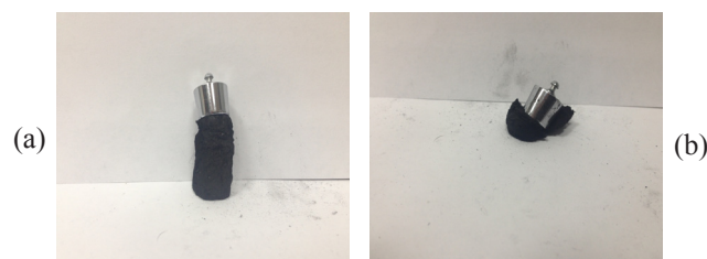
Fig. 5. a – picture of aerogel based on ECR CVD graphene/MWCNTs/chitosan (weight-0.09 g) with loading of 10 g; b – picture of aerogel based on MWCNTs/chitosan (weight-0.085 g) with loading of 10 g.
