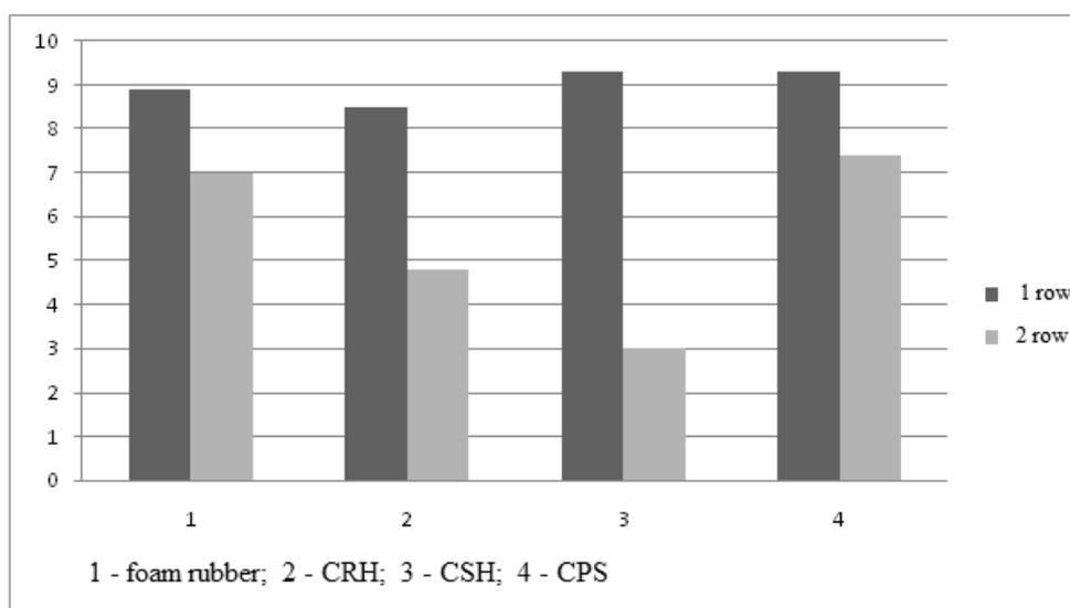
Fig. 4 – Comparative characteristics of sorbents: 1 row – oil collected at 0° C, 2 row – squeezed oil at room temperature.
