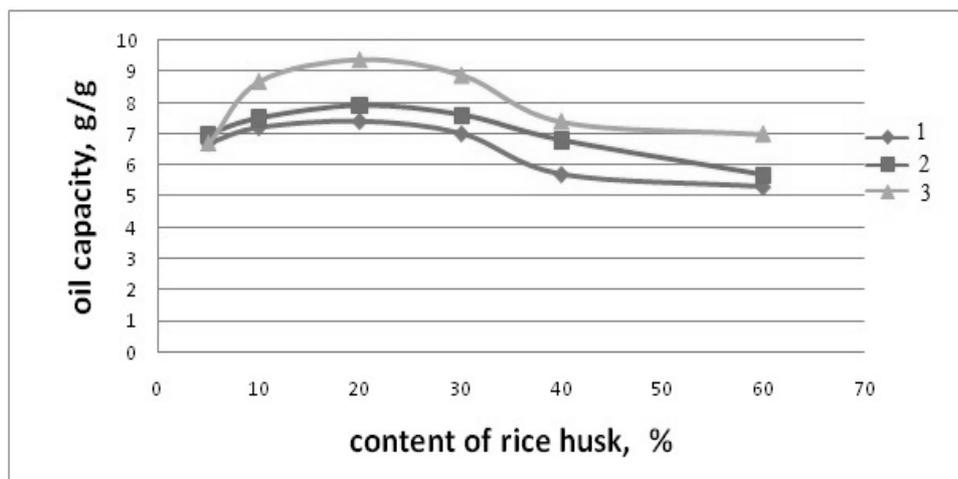
Fig. 3 – Effect of rice husk on oil intensity of carbon polystyrene sorbent (CPS) adsorbent at the various temperatures: 1 – oil capacity of CPS at temperature 0°C, 2 – oil capacity of CPS at temperature 10°C, 3 – oil capacity of CPS at temperature 25°C.
