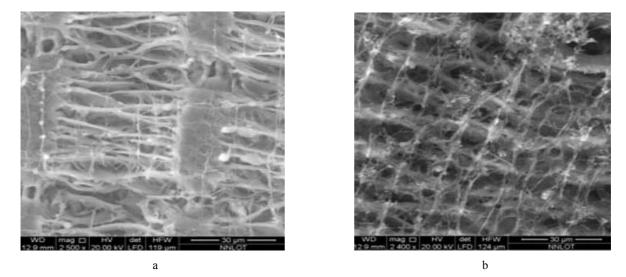
Fig. 2 – SEM pictures of the carbon-polystyrene material with excipients of RH 30% after the heat treatment: a – Carbon+polysterene+CRH (CPCRH400), b – Carbon+polysterene+CRH (CPCRH700).
