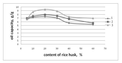
Fig. 3 – Effect of rice husk on oil intensity of carbon polystyrene sorbent (CPS) adsorbent at the various temperatures: 1 – oil capacity of CPS at temperature  $0^{\circ}$ C, 2 – oil capacity of CPS at temperature  $10^{\circ}$ C, 3 – oil capacity of CPS at temperature  $25^{\circ}$ C.
