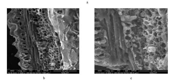
Fig. 1 – SEM photographs of RH: a – initial RH, b, c – after the heat treatment (at various increase).
