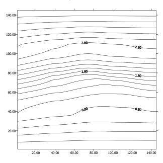
Fig. 8. Interaction of the wind turbine with the air flow ( $\omega=6$ )
