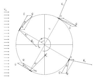
*Fig. 2.* Rotating counterclockwise by a working wind turbine blades
