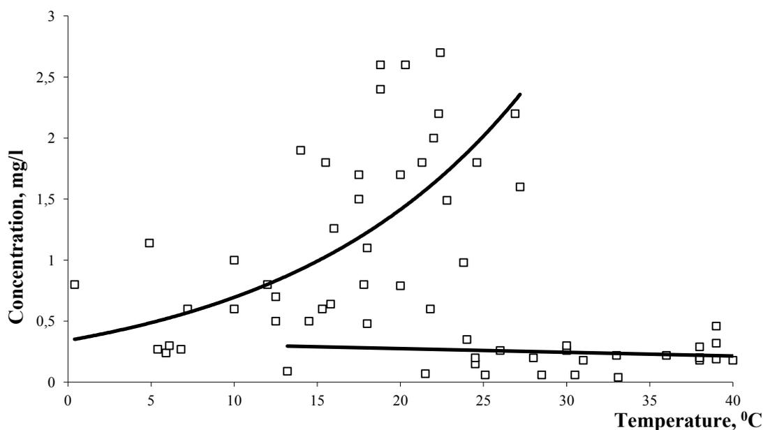
Figure 1 - The dependence of the oil content in the water on temperature of cooling reservoir Ekibastuz Power Plant-1
