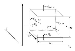
Fig.1 Control volume for the generalized transport equation [4], where  $\rho u \phi |_{i,i+\Delta i}$  – describes
