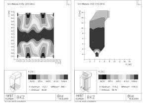
Fig.7 The temperature profile of the burners and in the longitudinal section of the combustion chamber
