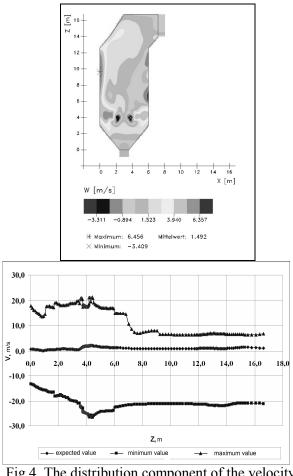
Fig.4 The distribution component of the velocity V in longitudinal section and the height of the combustion chamber
