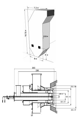
Fig.2 The general form of the combustion chamber and coal-dust burner
